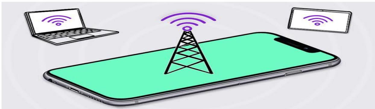
**Access point (wireless access point):** A wireless access point (WAP) is a networking device that allows a Wi-Fi compliant device to connect to a wired network. The WAP can either be physically connected to a router or be integrated into the router itself. A WAP is not a hotspot, which is the physical location where Wi-Fi access to a WLAN is available.
